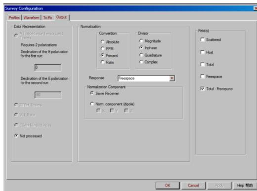
In the example above are the selections for a standard dipole-dipole FEM moving array. Here the data is to be normalized to the Inphase of the primary field and computed in units of Percent. The output fields are Total-Freespace and to the freespace of the same component as the data.
