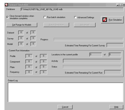
This interface provides controls to the super-engine which controls the modules which actually compute the synthetic responses. It provides progress reports in the middle section and in the white box to the bottom, information useful to the developers.
