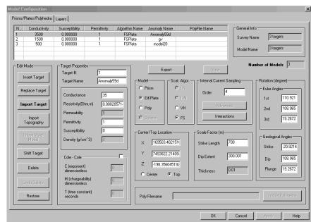
The other tab in the modelgui is for the insertion/editing/deletion/viewing of 3D anomalies.
