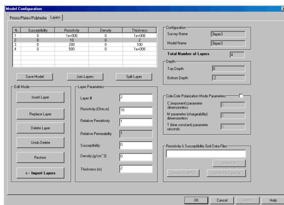
Layers can be defined by the resistivity, thickness, electrical permittivity, magnetic susceptibility and density. Also, the layers can be made polarizable through setting Cole-Cole parameters which is applicable for all EM modeling. The top layer is an air layer by default but can be set with suitable parameters for other applications such as marine or underground. For example, for surveys on the seabed one might set the top layer to be the conductivity of sea water.
